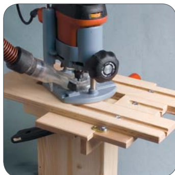
1) Routing with routing-jig and routing machine.
