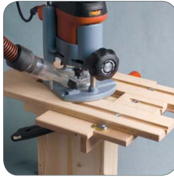
1) Routing with routing-jig and routing machine.
