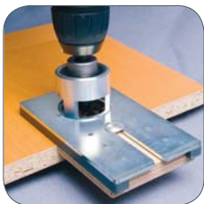
1) Drilling with jig
