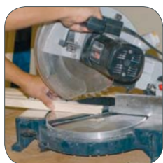
1) Cut to size glass bar and FIXclip-Profile
