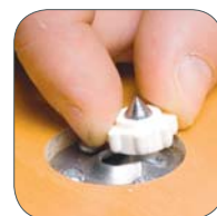
3) Transfer with the center punch
