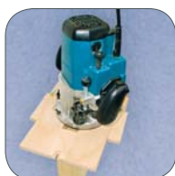
1) Route with routing-jig
