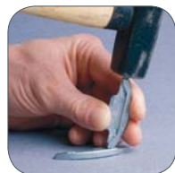
2) Bending locking clips
