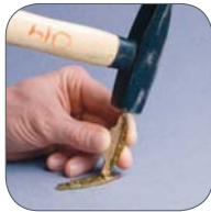
2) Bending locking clips
