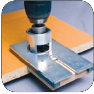
1) Drilling with jig
