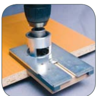
1) Drilling with jig
